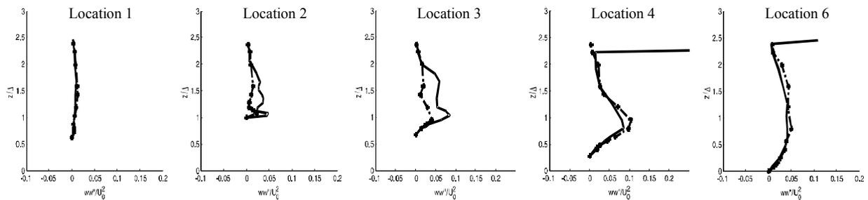
FIG. 9(B). REYNOLDS NORMAL STRESS ( $WW$ ) RESULTS OVER VARIOUS POSITIONS (NON-VEGETATED CASE SHOWN BY DOTTED LINE AND SOLID LINE INDICATES VEGETATED CASE WITH  $Q=25$  L/SEC) [ $ww'/u_o^2$  represents normalized Reynolds normal stresses whereas  $z/\Delta$  shows normalized depth of flow with reference to weir height ( $\Delta$ )]
