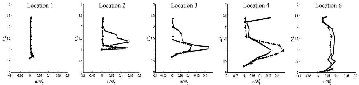
FIG. 9(A). REYNOLDS NORMAL STRESS ( $UU$ ) RESULTS OVER VARIOUS POSITIONS (NON-VEGETATED CASE SHOWN BY DOTTED LINE AND SOLID LINE INDICATES VEGETATED CASE WITH  $Q=25$  L/SEC) [ $uu'/u_o^2$  represents normalized Reynolds normal stresses whereas  $z/\Delta$  shows normalized depth of flow with reference to weir height ( $\Delta$ )]
