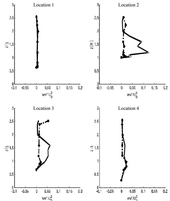
FIG. 8(C). REYNOLDS NORMAL STRESS ( $WW$ ) RESULTS OVER VARIOUS POSITIONS (NON-VEGETATED CASE SHOWN BY DOTTED LINE AND SOLID LINE INDICATES VEGETATED CASE WITH  $Q=40$  L/SEC) [ $ww''/u_0^2$  represents normalized Reynolds normal stresses whereas  $z/\Delta$  shows normalized depth of flow with reference to weir height ( $\Delta$ )]
