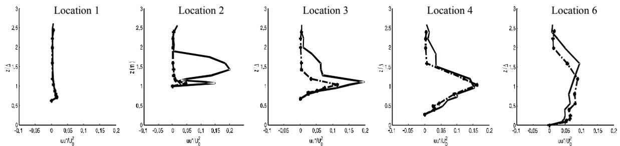
FIG. 10(A). REYNOLDS NORMAL STRESS ( $UU$ ) RESULTS OVER VARIOUS POSITIONS (NON-VEGETATED CASE SHOWN BY DOTTED LINE AND SOLID LINE INDICATES VEGETATED CASE WITH  $Q=40$  L/SEC) [ $uu'/u_o^2$  represents normalized Reynolds normal stresses whereas  $z/\Delta$  shows normalized depth of flow with reference to weir height ( $\Delta$ )]
