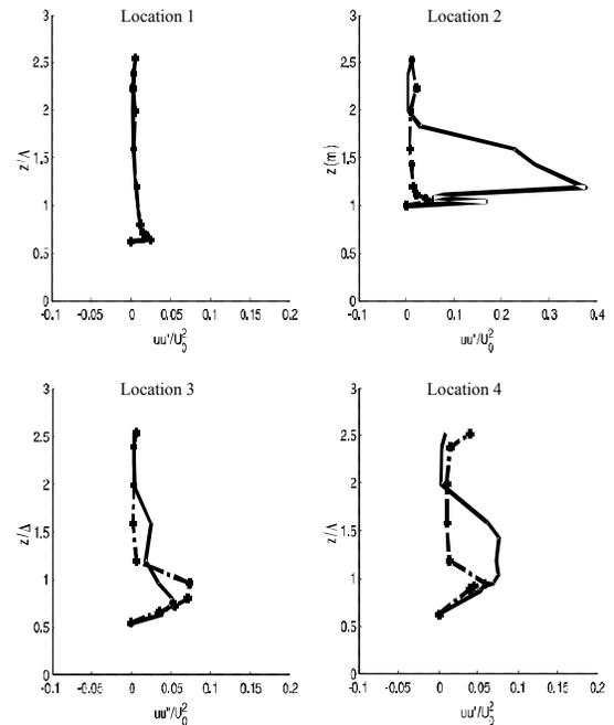
FIG. 8(B). REYNOLDS NORMAL STRESS ( $UU$ ) RESULTS OVER VARIOUS POSITIONS (NON-VEGETATED CASE SHOWN BY DOTTED LINE AND SOLID LINE INDICATES VEGETATED CASE WITH  $Q=40$  L/SEC) [ $uu''/u_0^2$  represents normalized Reynolds normal stresses whereas  $z/\Delta$  shows normalized depth of flow with reference to weir height ( $\Delta$ )]
