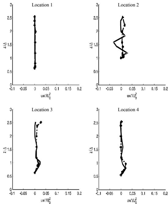
FIG. 8(A). REYNOLDS SHEAR STRESS RESULTS OVER VARIOUS POSITIONS (NON-VEGETATED CASE SHOWN BY DOTTED LINE AND SOLID LINE INDICATES VEGETATED CASE WITH  $Q=40$  L/SEC) [ $uw''/u_0^2$  represents normalized Reynolds shear stresses whereas  $z/\Delta$  shows normalized depth of flow with reference to weir height ( $\Delta$ )]
