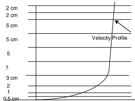
FIG. 6. MUTUAL DISTANCE ALONG THE DEPTH OF THE CHANNEL BETWEEN SUCCESSIVE POINTS OF VELOCITY MEASUREMENTS
