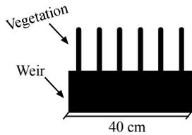
FIG. 3(B) CROSS-SECTIONAL VIEW OF THE WEIR CREST
