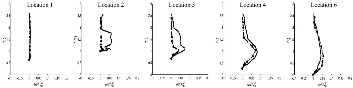
FIG. 10(B). REYNOLDS NORMAL STRESS (WW) RESULTS OVER VARIOUS POSITIONS (NON-VEGETATED CASE SHOWN BY DOTTED LINE AND SOLID LINE INDICATES VEGETATED CASE WITH  $Q=40$  L/SEC) [ $ww/u_o^2$  represents normalized Reynolds normal stresses whereas  $z/\Delta$  shows normalized depth of flow with reference to weir height ( $\Delta$ )]
