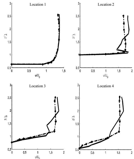
FIG. 7(A). PRIMARY VELOCITY RESULTS OVER VARIOUS POSITIONS (NON-VEGETATED CASE SHOWN BY DOTTED LINE AND SOLID LINE INDICATES VEGETATED CASE WITH  $Q=40$  L/SEC) [ $u/u_0$  represents normalized stream-wise velocity whereas  $z/\Delta$  shows normalized depth of flow with reference to weir height ( $\Delta$ )]
