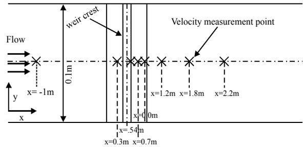
FIG. 5. LOCATIONS OF VARIOUS POINTS ALONG THE LENGTH OF THE CHANNEL SELECTED FOR DATA COLLECTION
