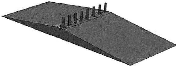
FIG. 3 (A). A 3D VIEW OF MODELLED WEIR AND VEGETATION IN THE CHANNEL
