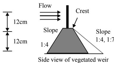
FIG. 4. WEIR WITH DIFFERENT LEeward SLOPES 1:4 AND 1:7
