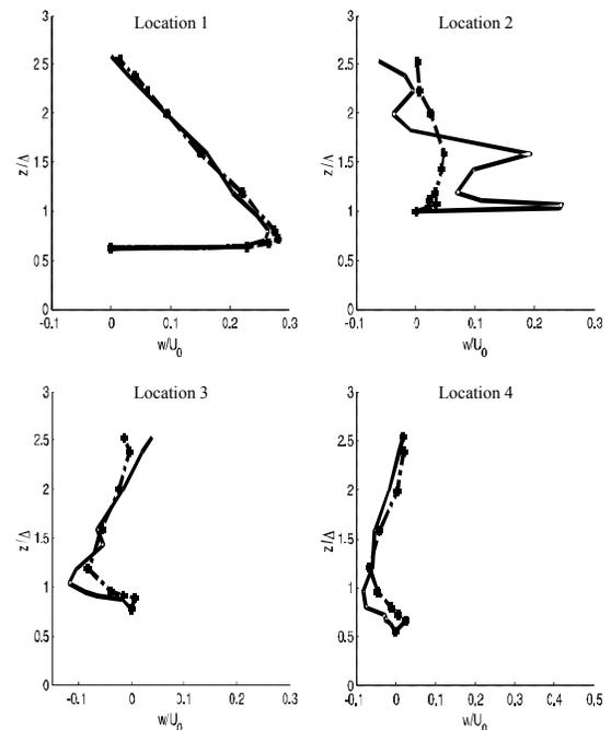
FIG. 7(B). VERTICAL VELOCITY RESULTS OVER VARIOUS POSITIONS (NON-VEGETATED CASE SHOWN BY DOTTED LINE AND SOLID LINE INDICATES VEGETATED CASE WITH  $Q=40$  L/SEC) [ $w/u_0$  represents normalized vertical velocity whereas  $z/\Delta$  shows normalized depth of flow with reference to weir height ( $\Delta$ )]
