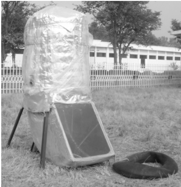
FIG. 3. FABRICATED SOLAR BIOGAS DIGESTER WITH FLEXIBLE GAS-HOLDER
