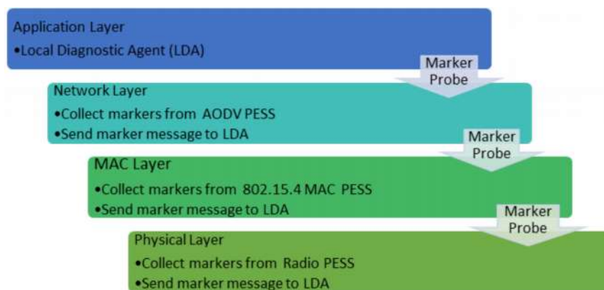
FIG. 2. LDA PERIODICALLY SENDS MARKER PROBE AFTER PROBE INTERVAL TO PROTOCOL STACK LAYERS
