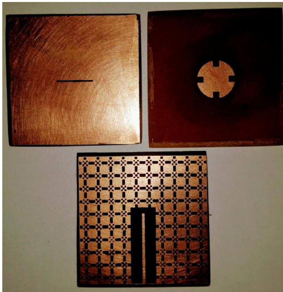
FIG. 9. FABRICATED PROTOTYPE OF THE PROPOSED ANTENNA WITH RADIATING ELEMENT, SLOT LINE AND EBG GROUND PLANE LAYERS
