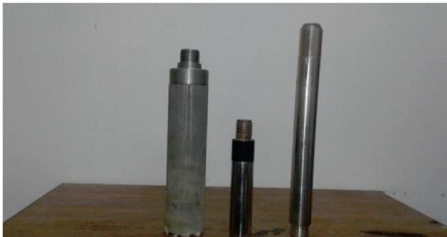
FIG. 1. PICTURE OF SHELBY TUBE ALONG WITH CONNECTORS
