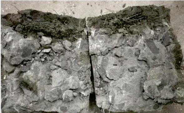
FIG. 8. PENETRATION OF WATER IN FA STEEL FIBERS REINFORCED CYLINDER
