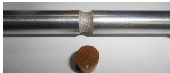
FIG. 2(b). COPPER ELECTRODE WITH PREPARED SPECIMEN
