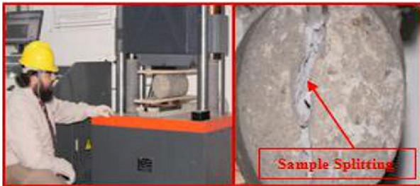
FIG. 17. SPLITTING TENSILE TEST ON CONCRETE CYLINDER
