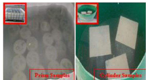
FIG. 7. TEST SPECIMENS CURED IN CHLORIDE MEDIUM
