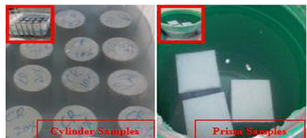
FIG. 8. TEST SPECIMENS CURED IN SULPHATE MEDIUM
