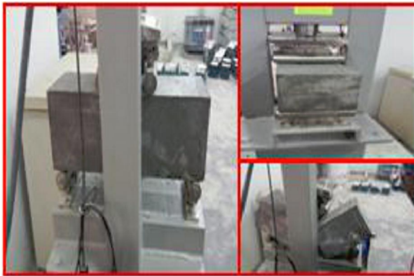
FIG. 14. FLEXURAL STRENGTH TEST OF CONCRETE PRISMS
