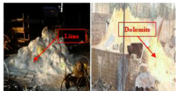
FIG. 5. FLUX MATERIALS ARE LEFT EXPOSED TO NATURE
