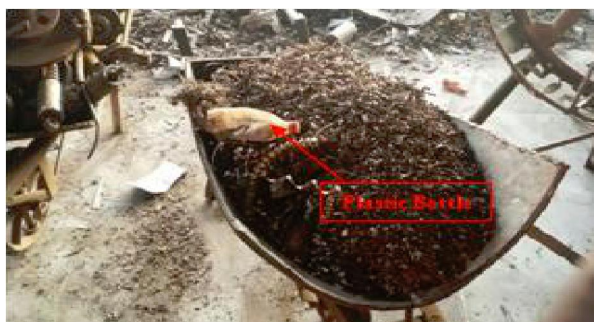
FIG. 2. NON-METALLIC ITEMS LEFT IN SCRAP METAL
