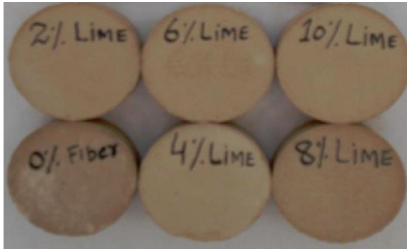
FIG.10. CLAYEY SAMPLE MIXED WITH LIME
