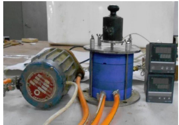
FIG. 4. SCHEMATIC REPRESENTATION OF THE THERMAL CONDUCTIVITY DEVICE IN OPERATION
