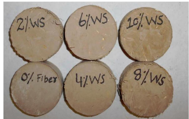
FIG. 7. CLAYEY SAMPLE MIXED WITH WHEAT STRAW
