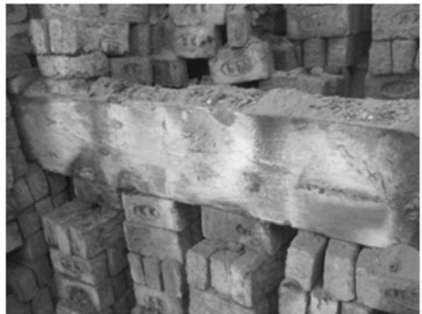
*FIG. 9. BEAMS WARPED DURING THE PROCESS OF COMMERCIAL BAKING*
