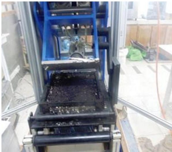
(a) COMPACTING SAMPLE BY ROLLER COMPACTOR
