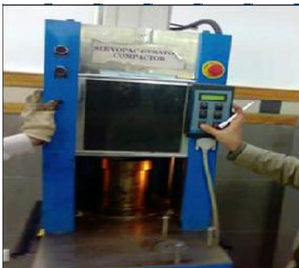
(c) COMPACTING SAMPLE BY GYRATORY COMPACTOR
