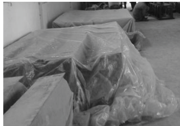
FIG. 4. MOIST CLAY BLOCKS WRAPPED WITH PLASTIC SHEET COVER ARE BEING DRIED IN SHADE
