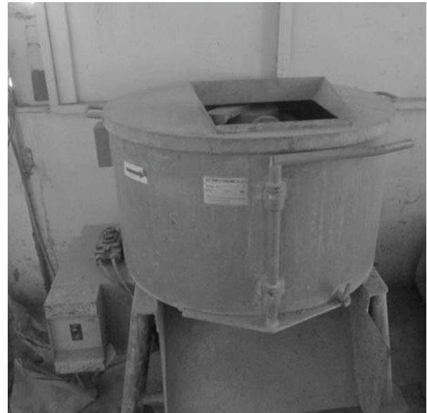
FIG. 1. PAN MIXER USED FOR MIXING OF CLAY PIT SAND AND WATER
