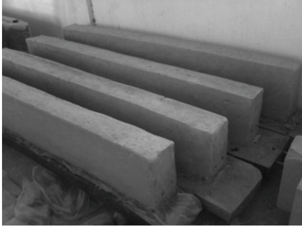
FIG. 5. A VIEW OF SUN-DRIED CLAY BLOCKS
