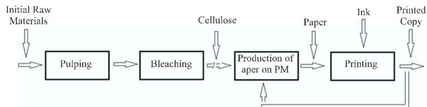
FIG. 1. SYSTEM APPROACH TO CONTROL PAPER-PRINTING CHARACTERISTICS
