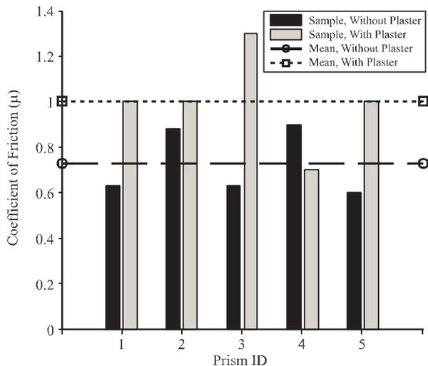
FIG. 13. COEFFICIENTS OF FRICTION OF TYPE-1 BLOCKS, WITH AND WITHOUT PLASTER
