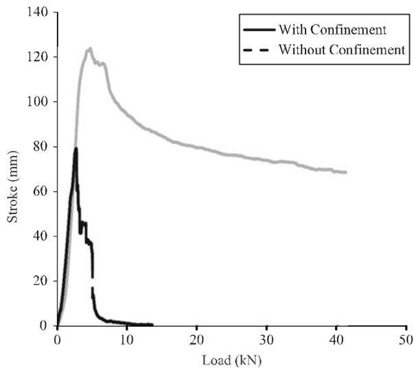
FIG. 12. LOAD DEFORMATION CURVE FOR THE SHEAR TEST OF A TRIPLET WITH PLASTER WITHOUT CONFINEMENT AND A TRIPLET WITH PLASTER WITH CONFINEMENT
