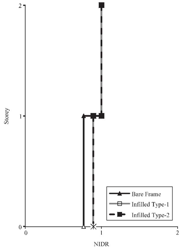
FIG. 19. NORMALIZED INTERSTOREY DRIFT RATIOS FOR THE TWO STOREYED FRAMES AT THE OCCURRENCE OF THE FIRST YIELD IN THE RESPECTIVE FRAMES
