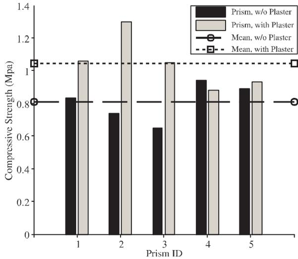
FIG. 6. COMPRESSIVE STRENGTHS OF MASONRY PRISMS OF TYPE-1 BLOCKS
