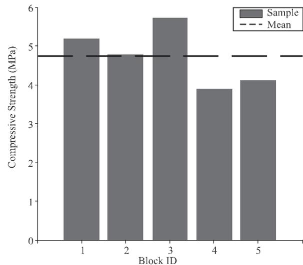
FIG. 3. COMPRESSION STRENGTHS OF TYPE-2 BLOCKS
