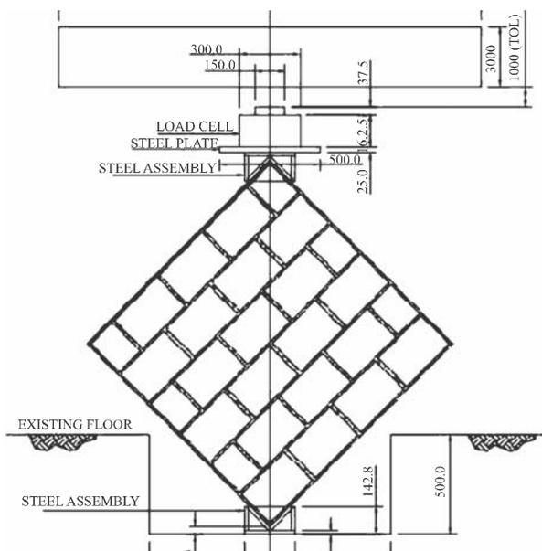
FIG. 15. SCHEMATIC DIAGRAM OF DIAGONAL COMPRESSION TEST SETUP SHOWING TOP & BOTTOM ASSEMBLY WITH LOAD CELL
