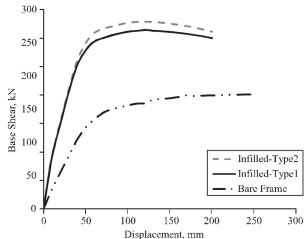
FIG. 21. PUSHOVER CURVE OF THE FOUR STOREYED RC FRAMES MODELLED FOR THREE SCENARIOS NAMELY I) BARE FRAME WITHOUT INFILL; II) INFILLED FRAME WITH TYPE-1 INFILL AND III) INFILLED FRAME WITH TYPE-2 INFILL
