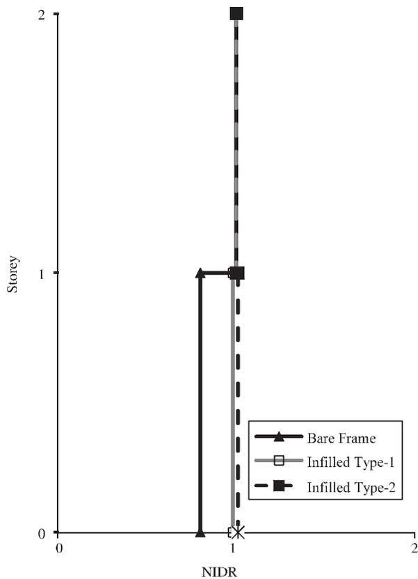
FIG. 20. NORMALIZED INTERSTOREY DRIFT RATIOS FOR THE TWO STOREYED FRAMES AT THE OCCURRENCE OF THE MAXIMUM BASE SHEAR IN THE RESPECTIVE FRAMES
