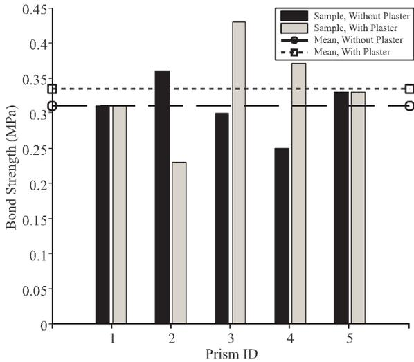
FIG. 10. BOND STRENGTHS OF MASONRY TRIPLETS OF TYPE-2 BLOCKS, WITH AND WITHOUT PLASTER
