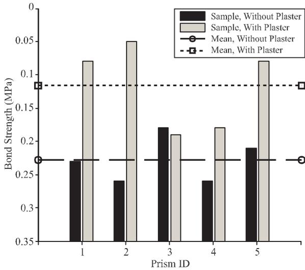
FIG. 9. BOND STRENGTHS OF MASONRY TRIPLETS OF TYPE-1 BLOCKS, WITH AND WITHOUT PLASTER
