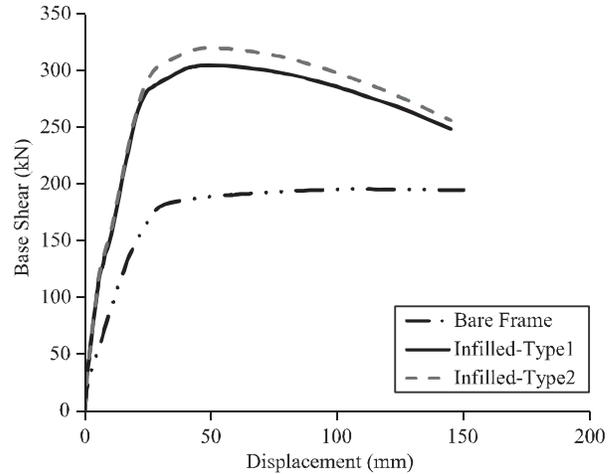
FIG. 18. PUSHOVER CURVE OF THE TWO STOREYED RC FRAMES MODELLED FOR THREE SCENARIOS NAMELY I) BARE FRAME WITHOUT INFILL; II) INFILLED FRAME WITH TYPE-1 INFILL AND III) INFILLED FRAME WITH TYPE-2 INFILL
