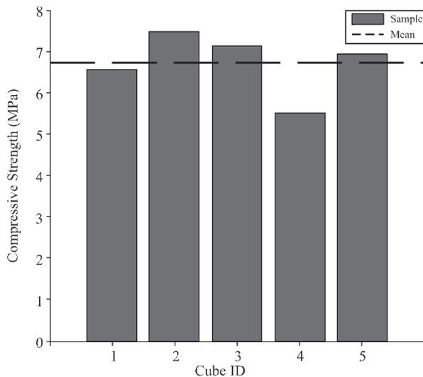
FIG. 4. COMPRESSIVE STRENGTHS OF MORTAR CUBES
