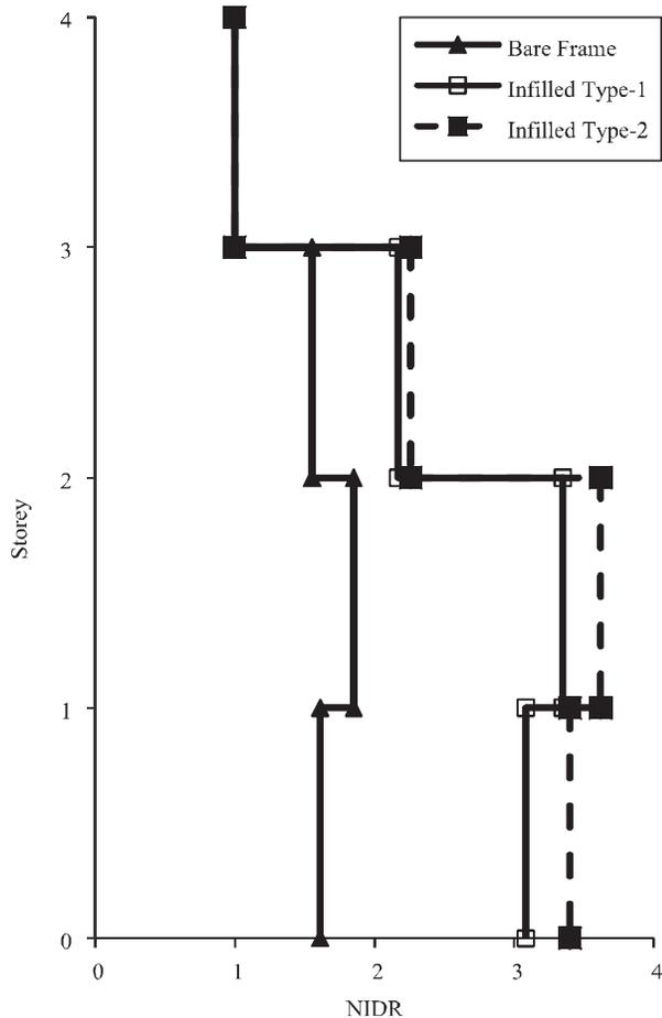
FIG. 22. NORMALIZED INTERSTOREY DRIFT RATIOS FOR THE FOUR STOREYED FRAMES AT THE OCCURRENCE OF THE FIRST YIELD IN THE RESPECTIVE FRAMES
