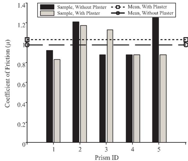
FIG. 14. COEFFICIENTS OF FRICTION OF TYPE-2 BLOCKS, WITH AND WITHOUT PLASTER
