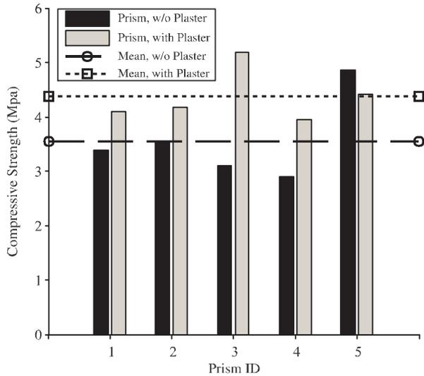
FIG. 7. COMPRESSIVE STRENGTHS OF MASONRY PRISMS OF TYPE-2 BLOCKS
