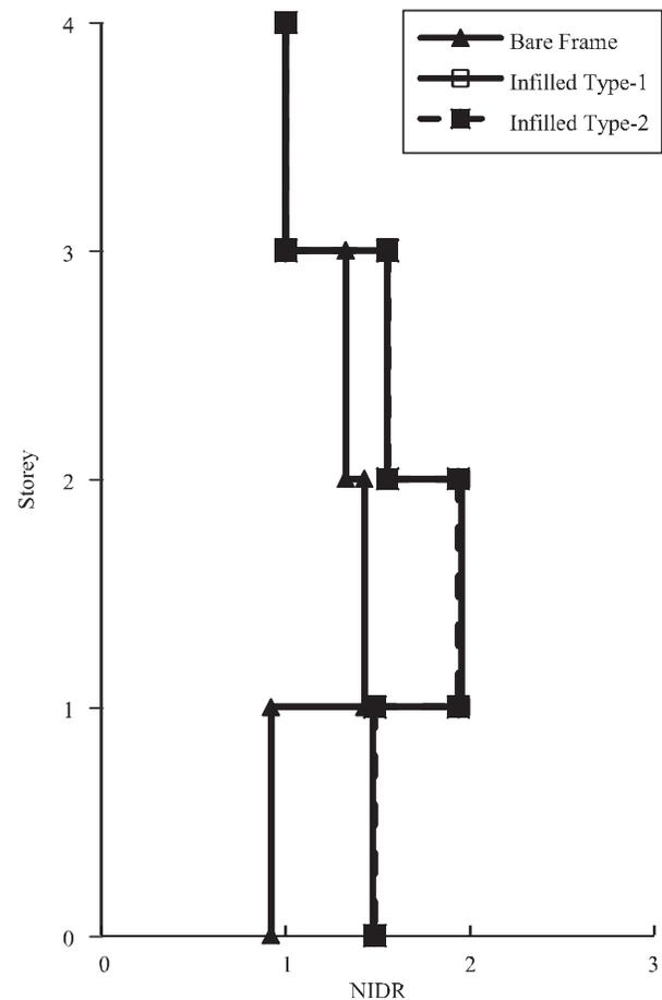
FIG. 23. NORMALIZED INTERSTOREY DRIFT RATIOS FOR THE FOUR STOREYED FRAMES AT THE OCCURRENCE OF THE MAXIMUM BASE SHEAR IN THE RESPECTIVE FRAMES
