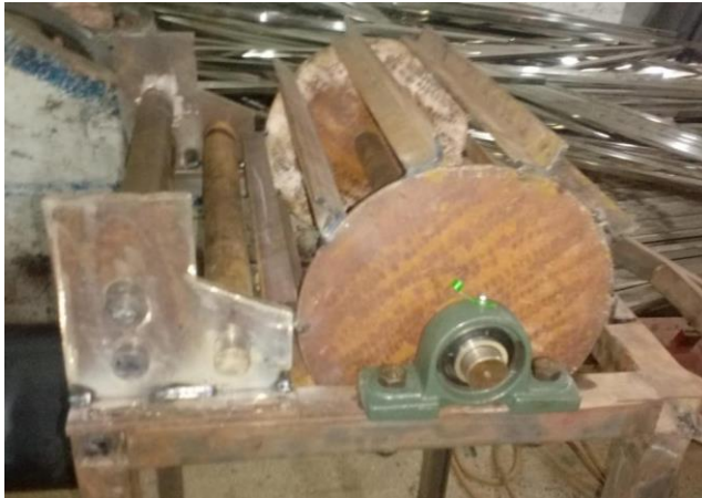
Fig. 12 (b). Side view of Fabricated Roller Drum
