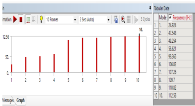
Fig. 8. 10 Modes Shape Frequencies Of Frame From Modal Analysis
