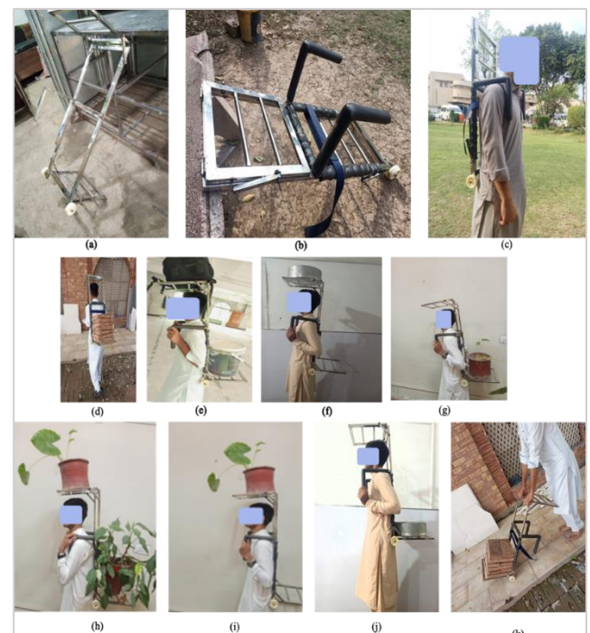
Fig. 6. Fabricated Toolkit And Its Utilization Of Toolkit By Workers For Various Loading In Various Modes, (a) Toolkit After Welding And Wheel Assembly, (b) Toolkit After Cushioning And Belt Installation, (c) Toolkit In Inactive-Mode (Closed Top And Bottom Surfaces), (d) Transportation Of Bricks By Worker In BLM, (e) Paint Box And Filled Bag Carried By A Worker In CLM, (f) Steel Pot Carried By Worker In OLM, (g) Flowerpot Carried By Worker In BLM, (h) Flowerpots Carried By Worker In CLM, (i) Flower Pot Carried In OLM, (j) Steel Pot Carried In BLM, (k) Bricks Transportation In TM.
