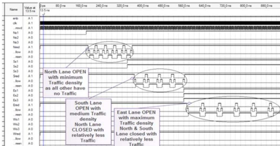
FIG. 7. RESPONSE TO DIFFERENT TRAFFIC DENSITY LEVELS
