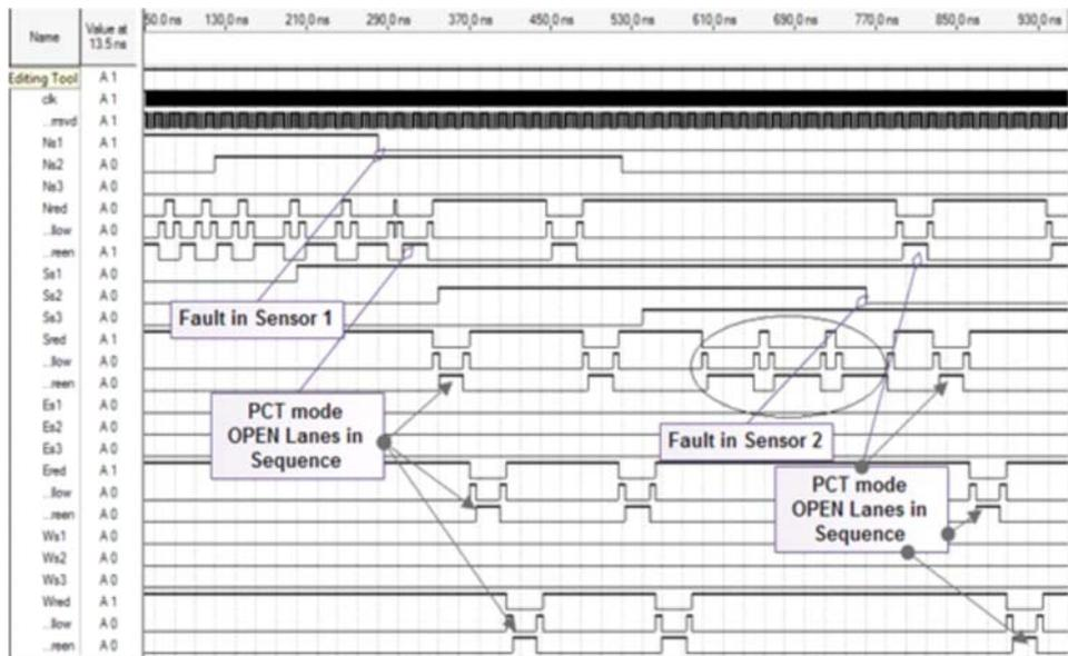
FIG. 8. SYTEM RESPONSE OVER DIFFERENT FAULT CONDITIONS
