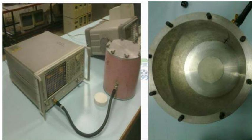
FIG. 9. NETWORK ANALYZER MEASUREMENT SETUP
