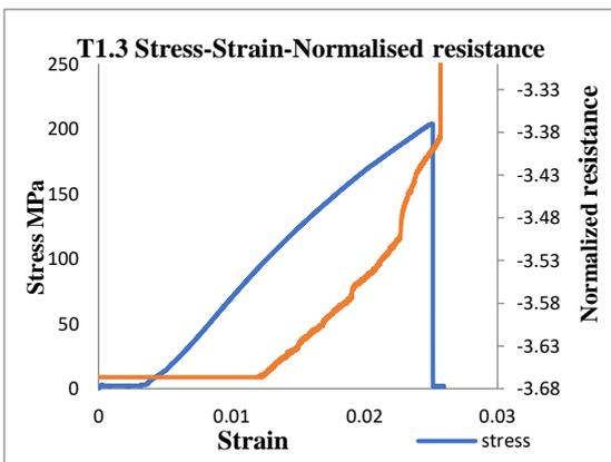
**Fig. 4(c).** T1.3 Stress-Strain-Normalized-Strain-Curve
