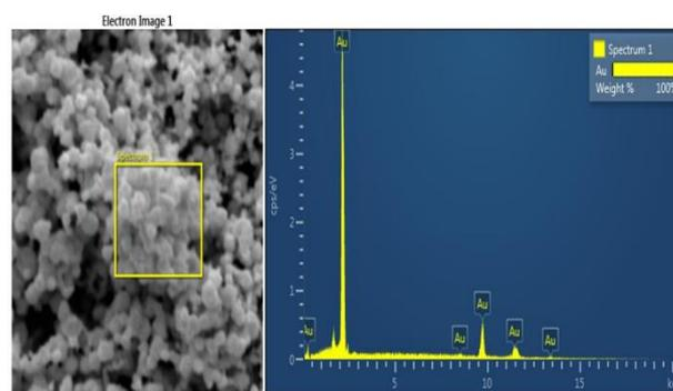
Fig. 1. SEM-EDS Image of AuNPs
