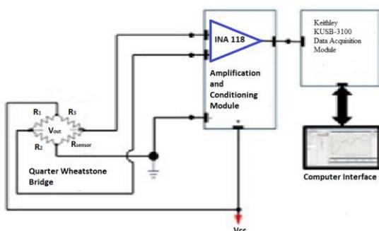
**Fig. 3(a).** SHM Set Up Circuit Diagram
