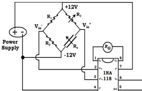
**Fig. 2(a).** Circuit Diagram of Wheatstone Bridge With Amplifier INA 118
