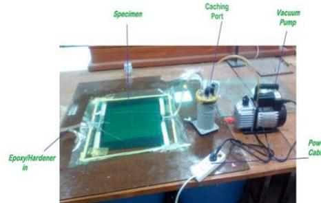
Fig. 2. Vacuum Bagging Set-Up
