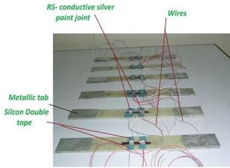
**Fig. 3.** GFRP Specimen
