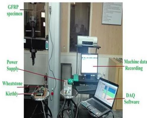
**Fig. 2(b).** Keithley With Wheatstone Bridge and Amplifier
