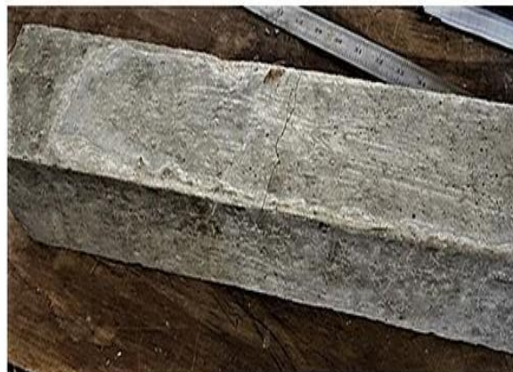
Fig. 5. Failure Cracks in Coir Fiber Reinforced Beam
