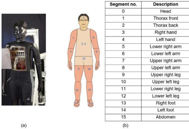
Fig. 5. (a) Thermal manikin "CHARLIE", (b) segmental representation of thermal manikin
