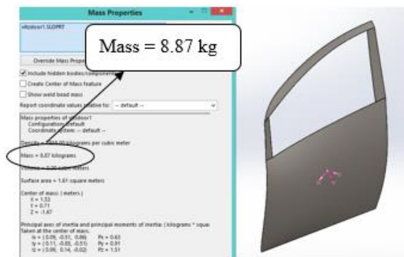
Fig. 10. Front Door, The Applied Material Is Carbon Steel ( t = 1.4 mm)
