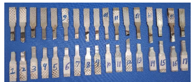
Fig. 15. Fractured tensile specimens
