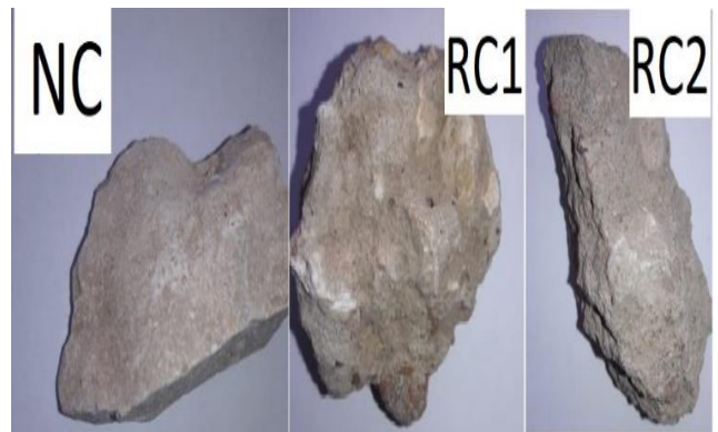
Fig. 8. Surface Texture Of Coarse Aggregates
