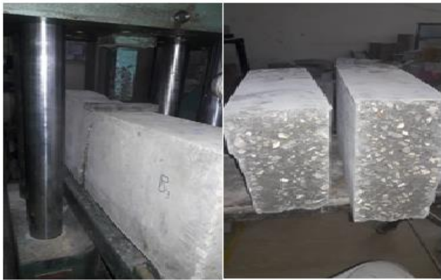
Fig. 19. Beam Specimen Testing
