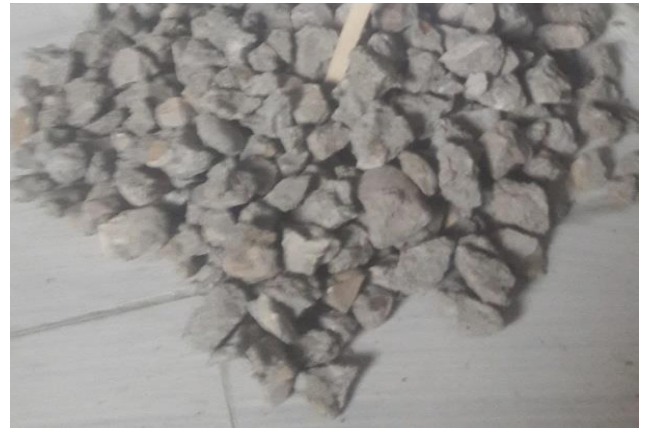
Fig. 7. Recycled Aggregates (Max. 25 Mm)
