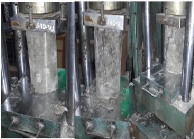
Fig. 9. Compressive Strength Test
