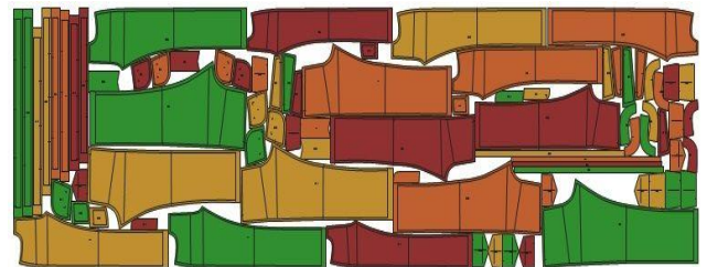
Fig. 6.a Trouser marker layout at 2% warp and 8% weft direction shrinkage
