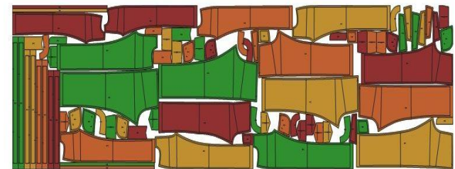
Fig. 6.b Trouser marker layout at 2% warp and 10% weft direction shrinkage
