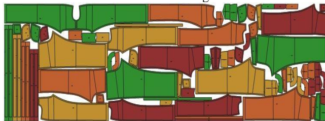
Fig. 6.c Trouser marker layout at 2% warp and 12% weft direction shrinkage
