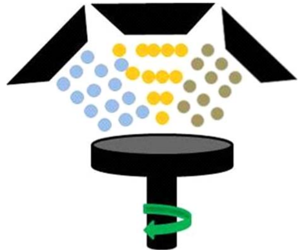
FIG. 1. SKETCH OF MAGNETRON SPUTTERING WITH THREE MAGNETRONS. SAMPLE IS PLACED UNDER THESE TARGETS AND ROTATING WITH CONSTANT SPEED
