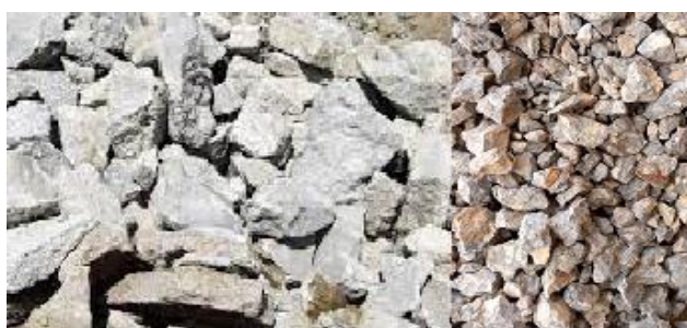
Fig. 2. Demolished Waste and Recycled Aggregates
