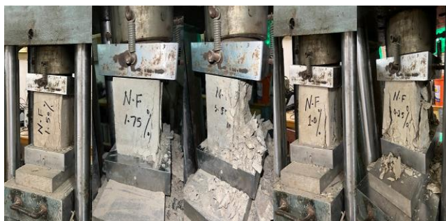
Fig. 5. Testing For Compressive Strength
