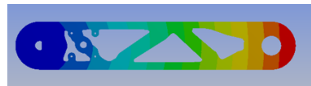
Fig. 13. Total Deformation of Optimized Link-2
