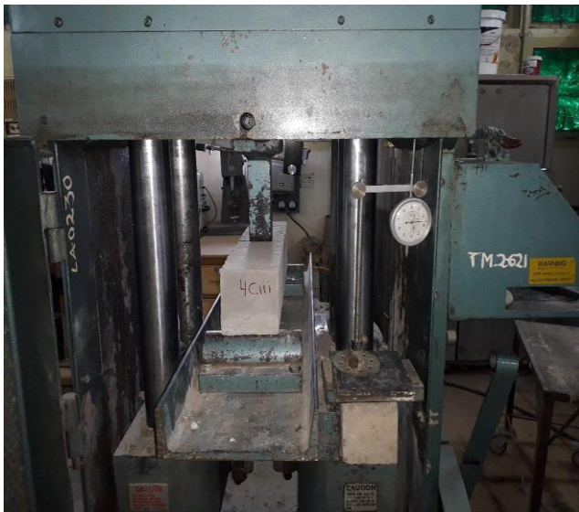
Fig. 7. Beam Loaded in UTM with Deflection Meter
