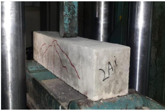
Fig. 4. Beam Loaded in UTMs
