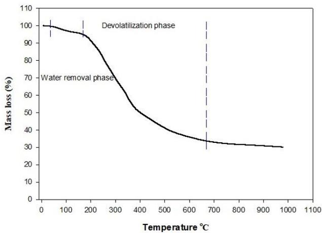
Fig. 8. TGA analysis of the collected particulates
