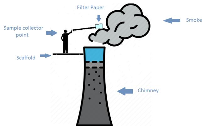
Fig. 4. Collecting samples from the exhaust.
