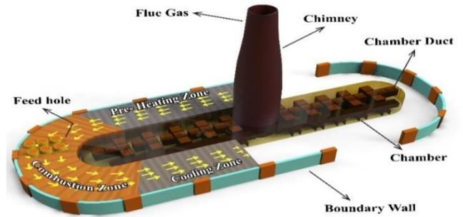
**Fig. 2.** An illustration of the fixed chimney bull's trench kiln's (FCBTK) layout, showing how the main trench is connected to tubular chambers.
