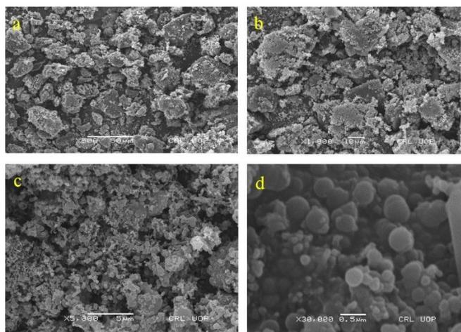
**Fig. 5.** SEM micrograph of the airborne particles at 500x, 1000x, 5000x, and 30000x magnifications (d).
