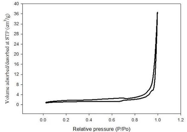
**Fig. 7.** Nitrogen adsorption at a temperature of -195 °C (isothermal curve).
