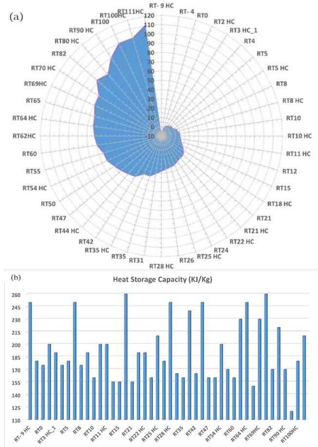
**Fig. 1.** RT PCM Comparison (a) Melting Point, (b) Heat Storage Capacity
