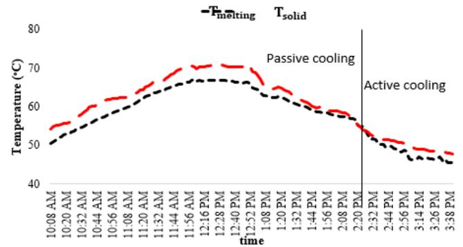
**Fig. 11.** Variation in temperature after active cooling in standard and modified PV panels
