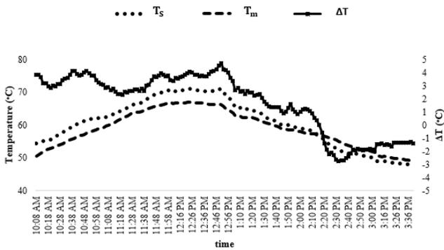
**Fig. 8.** Variation of the temperature of standard and modified PV panels during an extremely hot day
