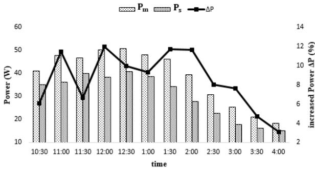
Fig. 5. Power comparison of both solar panels and percentage increase in output power
