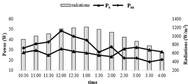
**Fig. 9.** Variation in Power of standard and modified PV panels during an extremely hot day
