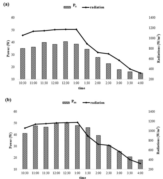
**Fig. 4.** Variation of the output power of PV panels at different radiations (a) Standard panel (b) Modified panel
