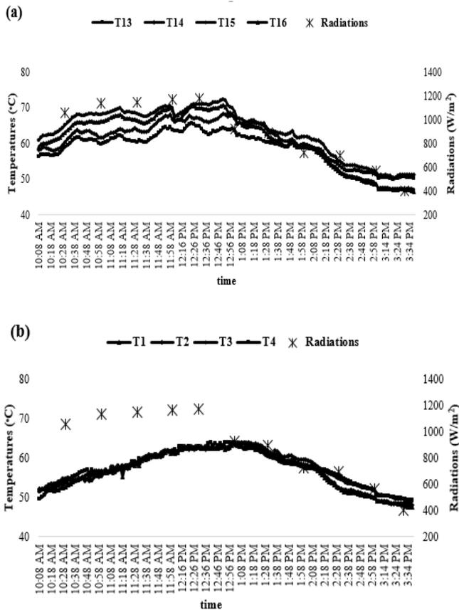
**Fig. 3.** PV panel surface temperature variations for different radiations (a) Standard panel (b) Modified panel
