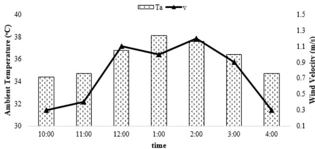
**Fig. 1.** Variation of ambient temperature and wind velocity throughout the experimentation
