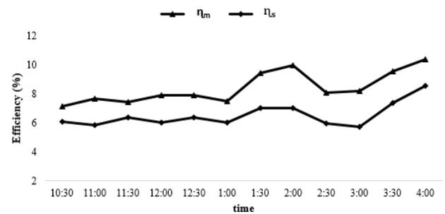
Fig. 7. Comparison of efficiencies of standard and modified PV panels
