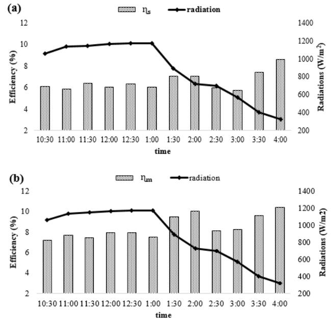
Fig. 6. Variation of Efficiency of the solar panels for different solar radiations (a) Standard panel (b) Modified panel
