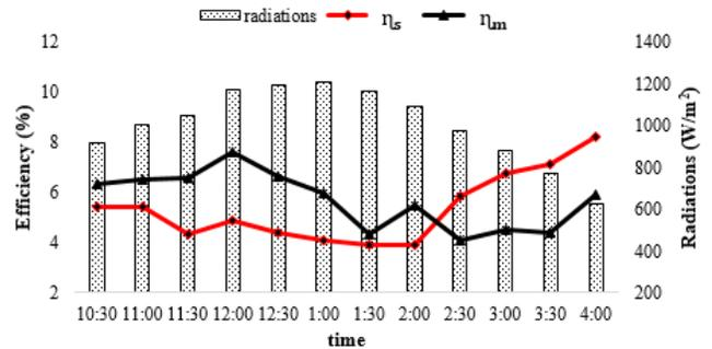
**Fig. 10.** Variation of Efficiency of standard and modified PV panels during an extremely hot day
