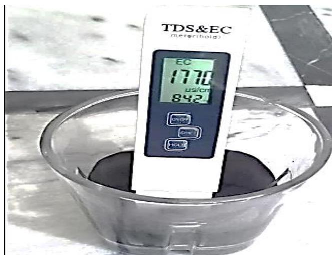
Fig. 6. Measuring electrical conductivity of different samples
