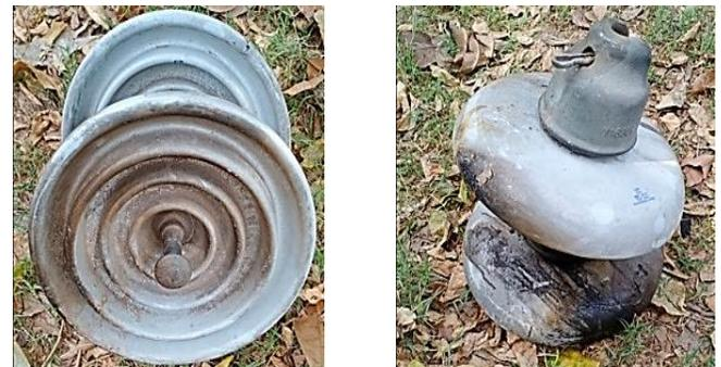
**Fig. 1.** Contaminated disc insulators
