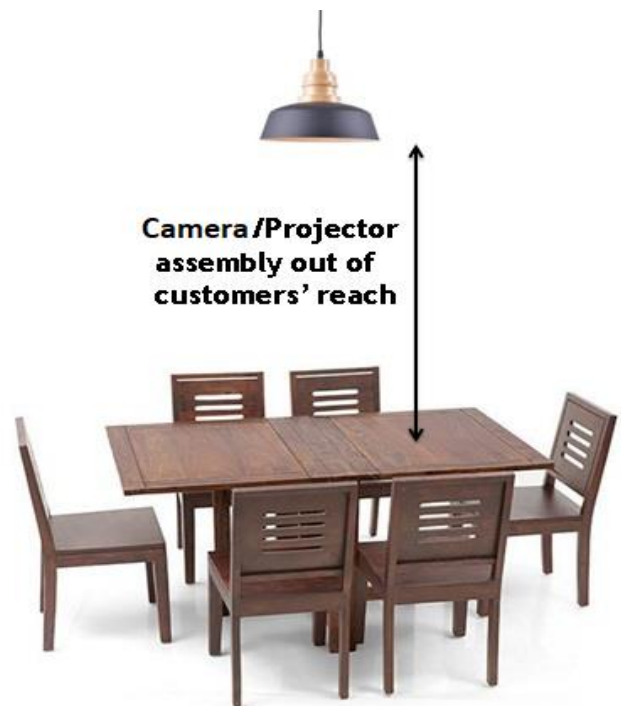
Fig. 4. Camera and projector holders
