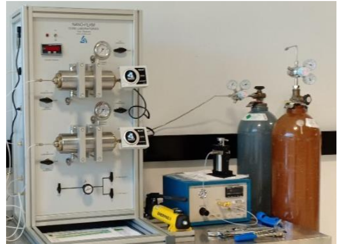
Fig. 2. Pictorial representation of the instrument for permeability and porosity measurements
