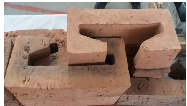
Fig. 2. Mortarless bricks with both ways interlocking system
