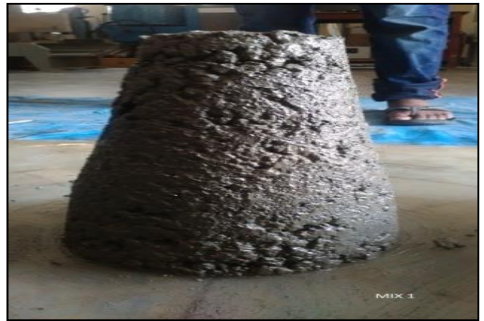
Fig. 7. Slump loss of CM 1
