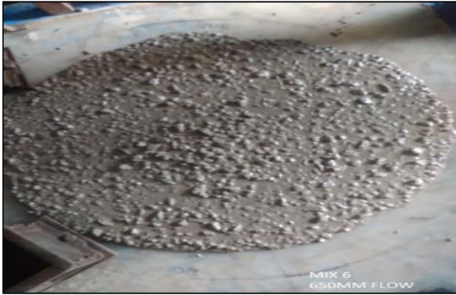
Fig. 8. Slump loss of CM 6
