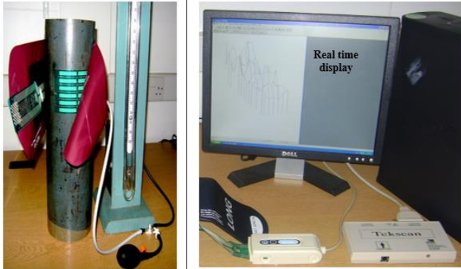
Fig. 2. Experimental setup for measurement of pressure at interface of cuff and metal cylinder
