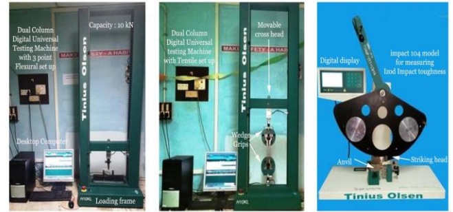
Fig. 2. Photographic image of Flexural, Tensile and Impact machine setup
