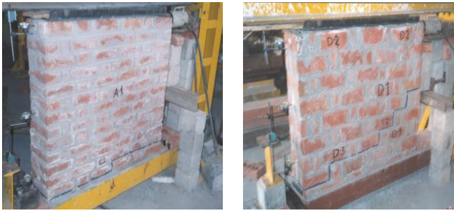
Fig. 4. Failure Pattern of RTB (left) and English bond (right) [23]
