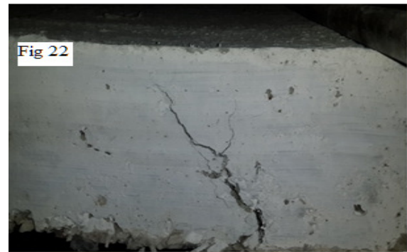
Fig. 22: Failure of slab S5 (10.0% MD) in flexure
