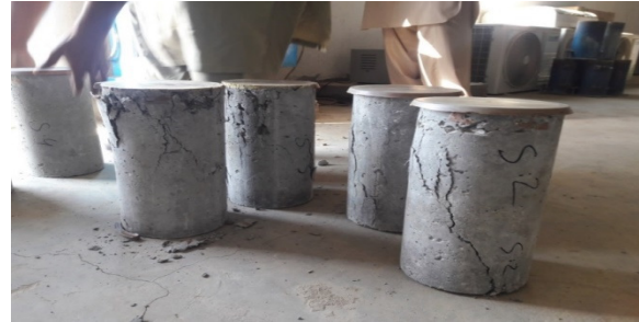
Fig. 7: Cylinder Specimens failure after compression test
