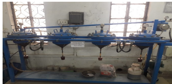
Fig. 10: Concrete water permeability apparatus
