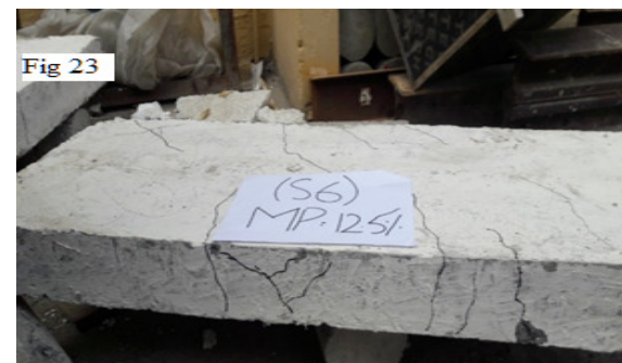
Fig. 23: Failure of slab S6 (12.5% MD) in flexure and shear
