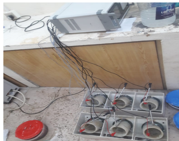
Fig. 27: Chloride ion migration test in progress
