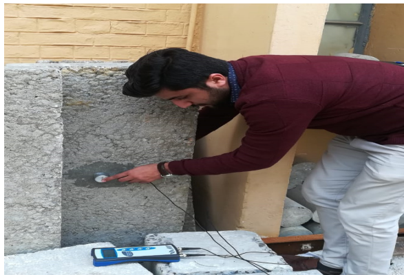
Fig. 25: UPV test being conducted on RCC slab specimen
