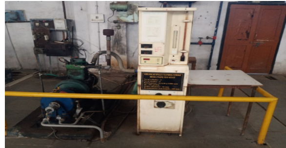
Fig. 1: Photograph of a 4-stroke CI Test-Setup
