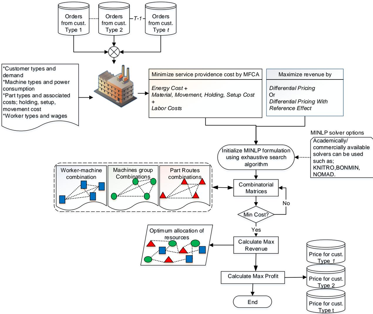
**Fig. 1.** Schematics of DP integrated with MFCA inspired costs
