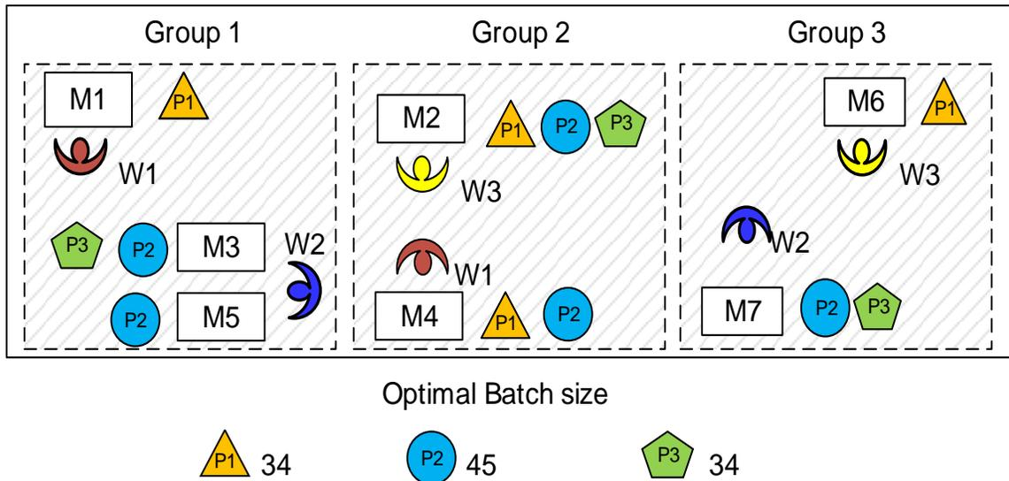
**Fig. 2.** Schematic representation of optimal resource grouping and batch size of parts to minimize the cost of service providence
