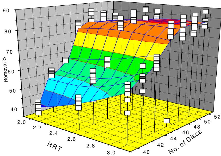
Fig. 3: Response Surface effect of Retention Time and Number of Discs on Removal of BOD<sub>5</sub>.
