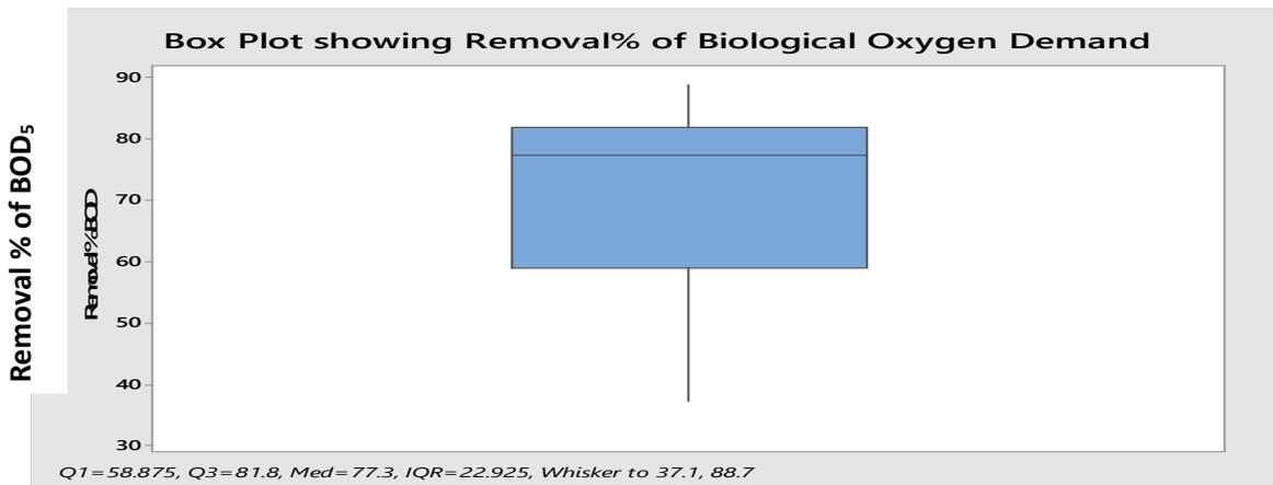
Fig. 2: Whisker Box Plot showing Removal% of BOD<sub>5</sub>, on 2, 2.5 and 3 Hours HRTs with different descriptive measures
