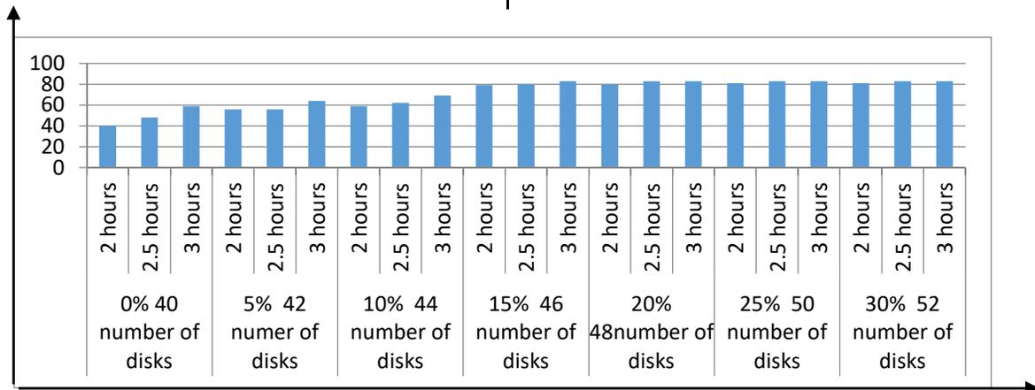
Fig. 1: Average removal of BOD<sub>5</sub> on different HRTs levels i-e; 2 hours, 2.5 hours and 3 hours with multiple numbers of discs
