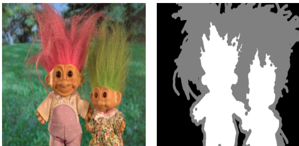
FIG. 1. A NATURAL IMAGE ALONG WITH A MANUALLY DEFINED TRIMAP
