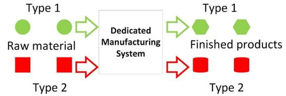
Fig. 1: DMS designed for multiple products
