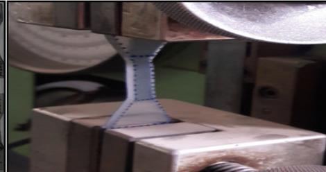
Fig. 8: Apparatus Setup of the Tensile Testing Specimen
