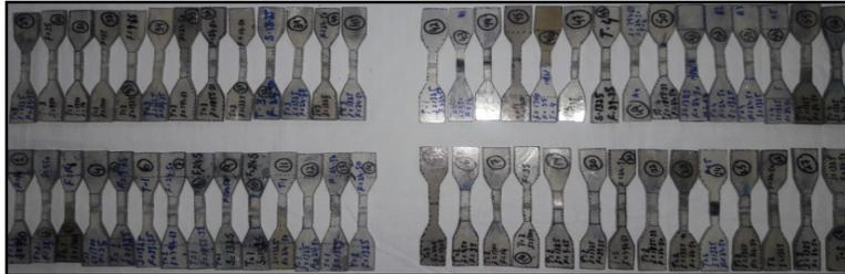
Fig. 7: Tensile Testing Specimens
