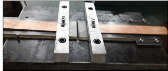
Fig. 4: Fixture for Clamping PC Plates
