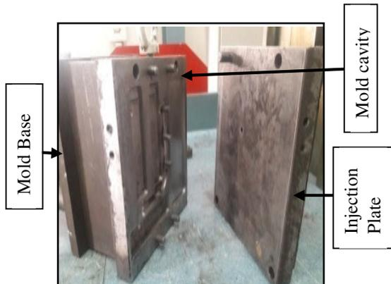
Fig. 3: Mold Assembly After Machining
