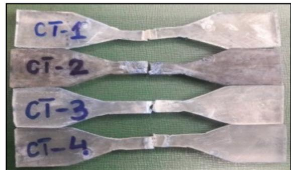
Fig. 18: Samples after Tensile Testing
