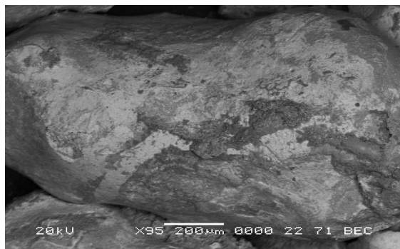
Fig. 14(a): Morphological results of Shikarap Iron Ore before Adsorption
