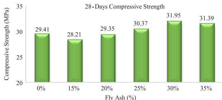
**FIG. 3. COMPRESSIVE STRENGTH OF 28-DAYS TEST RESULT WITH INCREASE OF FLY ASH**
