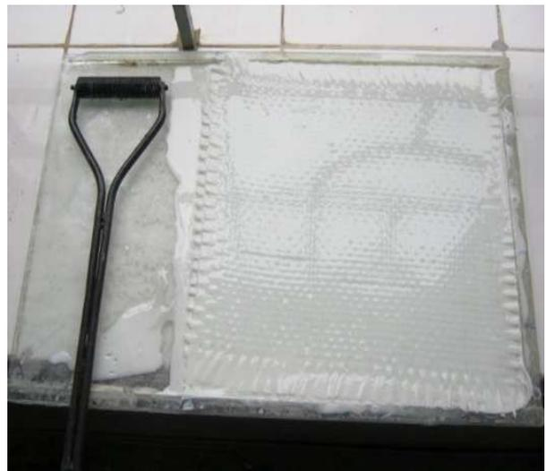
*FIG. 6. FIBER GLASS/EPOXY/ELO  $Sb_2O_3$ /CHLORINATED PARAFFINS/ COMPOSITES*
