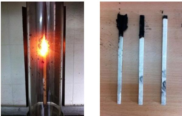
FIG. 1(A). IMAGE OF FIRE RETARDANT TEST ACCORDING TO LOI
