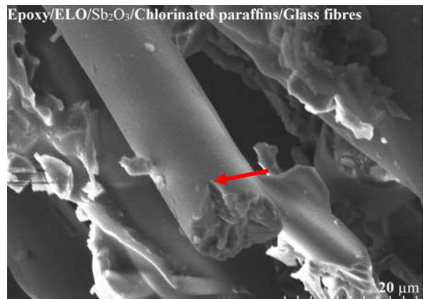
FIG. 10. FE-SEM MICROGRAPHS OF THE SAMPLES: COMPOSITES EPOXY/GLASS FIBRES AND COMPOSITES EPOXY/ELO/CHLORINATED PARAFFINS/GLASS FIBRES
